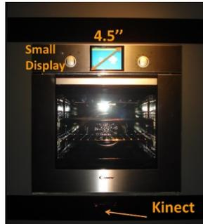
**Figure 1. Front view of MOTIC with the integrated small display and Kinect sensing device**
