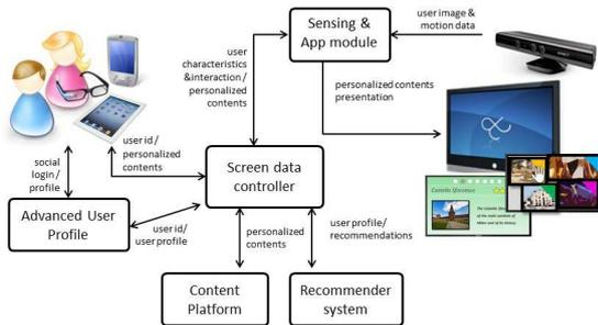
Figure 1: StreetSmart System Architecture.
